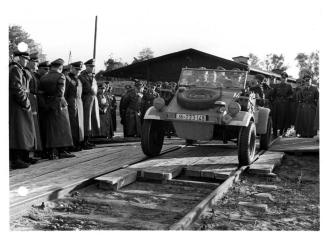
In 1943, Rüstsätze, or upgrade kits for VW Kubelwagen Types 82 and 87 were developed, which would make them schienengängig or railgoing. This conversion, designated VW Type 157, consisted of discs that were fitted to the insides of the regular road wheels. Spacers were added as necessary to match the track gauge. Thus the tires sat on the rails, providing propulsion, and they were kept on the track by the discs.
