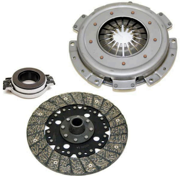
Common post 1971 clutch kit with proper component compatibility.
