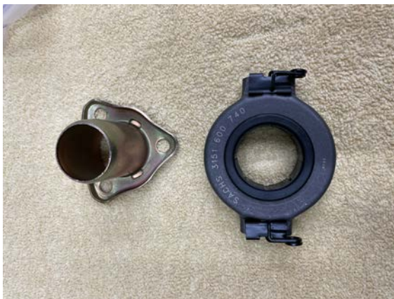
Here's an important photo. This shows the early release bearing with matching operation shaft compared to the later arrangement. Note the lack of the support sleeve with the early unit, and the difference in the shaft. (photo credit Clyde Maddox)
