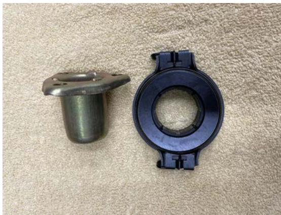
Here's the guide sleeve removed from the late transaxle for a better view. The release bearing we used as a reference. (Photo credit Clyde Maddox)
