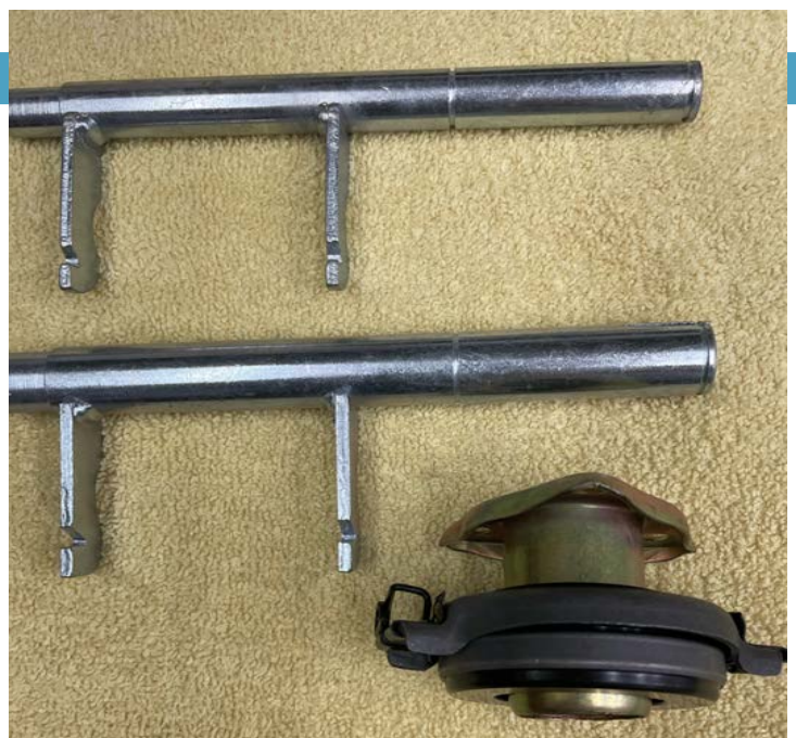
Two slightly different clutch operation shafts, with their matching late style release bearing. This release bearing is known as the "165B" as this is the suffix of the part number. Note the support sleeve that would normally be fitted to the late versions of the T1 transaxle to act as a release bearing guide. (Photo credit to Clyde Maddox)
