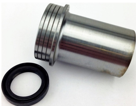
This adapter sleeve allows an early transaxle to be fitted with a late release bearings, and clutch operation shaft, as well as a late pressure plate. This piece is available from various retailers and works very well to bring an early transaxle up to par with later parts. The original input shaft seal is removed, and this sleeve (which incorporates its own input shaft seal) is pressed into place. These are a great way to have later, stronger parts in an early transaxle. (Photo credit Aircooled.net)
