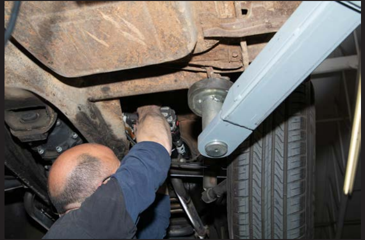
Frank drills a 1 ¼ inch hole in the front engine cover plate tin for the rear compressor brace; a special nut is provided.
