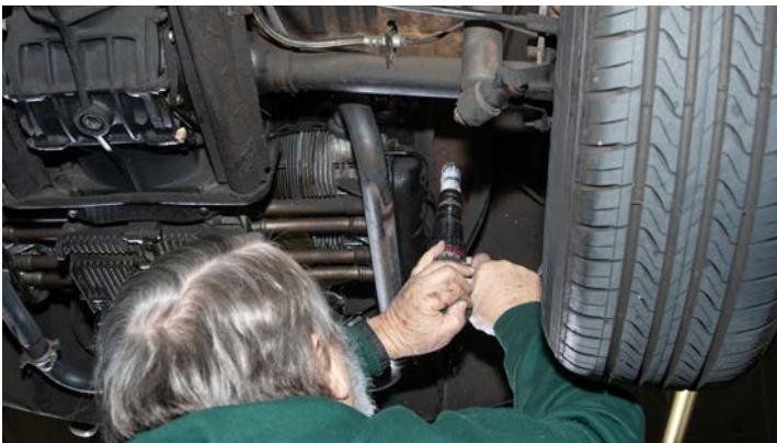
Two 1 ¼ inch holes are needed on the left side of the engine compartment for hose access. These are protected with grommets.
