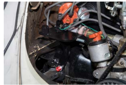
The compressor stand is installed, using specialized, color-coded hardware.
