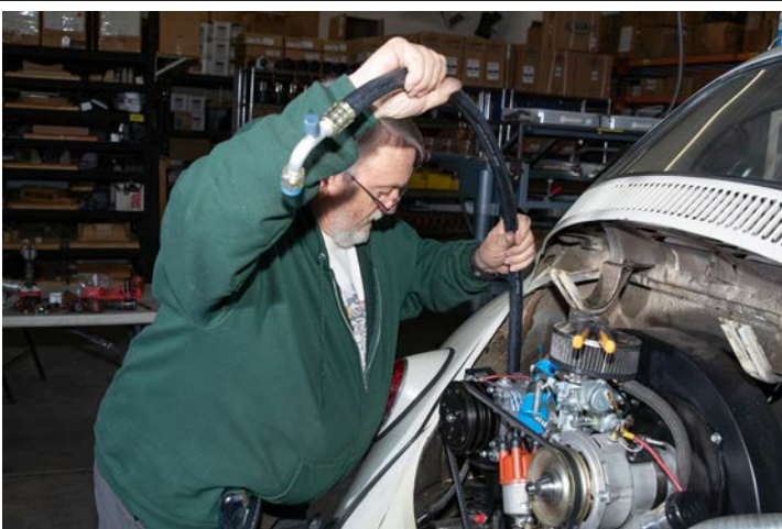
High-pressure hoses are fed from the engine compartment through the tin and attached to the compressor.
