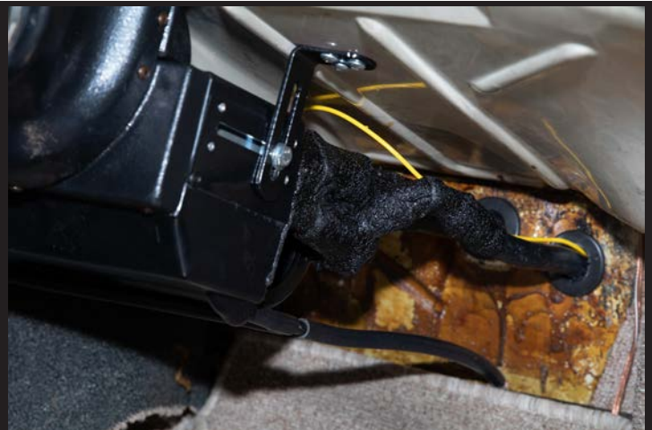
Final wiring for the evaporator is completed, and cork tape is wrapped on the metal fittings of the unit.
