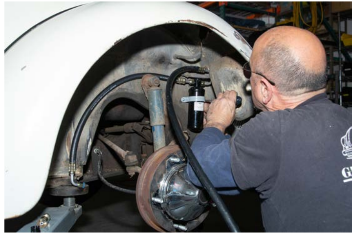
Frank removes the front passenger wheel and installs the dryer unit and installs the high-pressure hoses.
