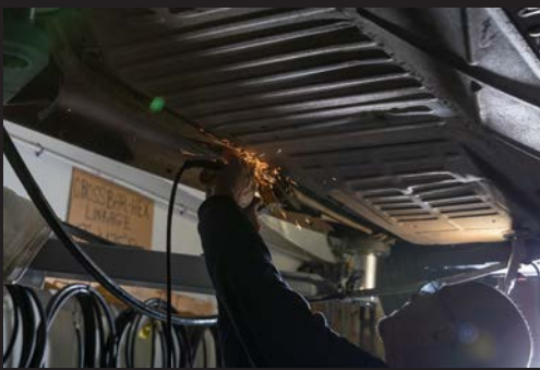
Before affixing the pressure hoses to the body, the original body seal nails must be removed one-by-one using a grinder. The hoses can then be attached using clamps along the channels.
