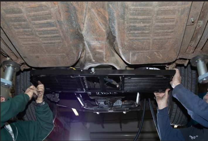
A dual-fan condenser mounts directly to the spring plate covers. The lower bolts are removed completely, while the others are only loosened slightly for the cover to open enough to receive the condenser.
