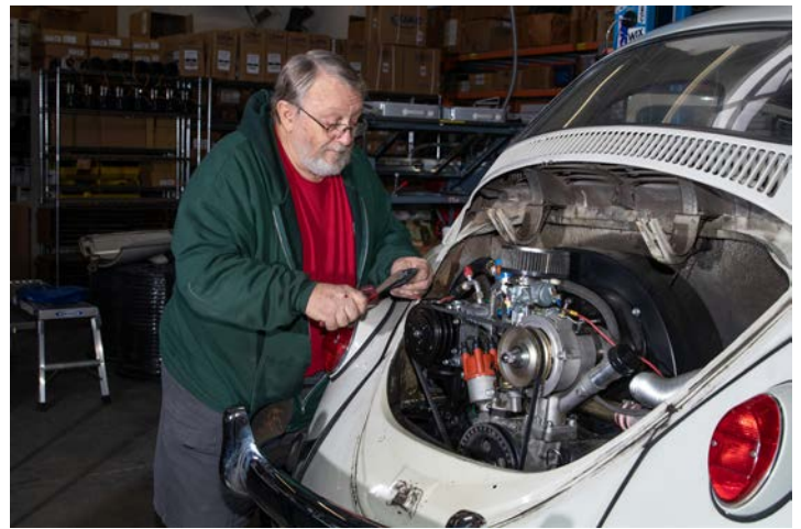
The remaining condenser wiring is completed.
