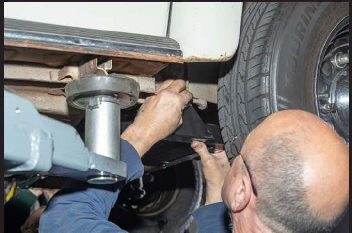
A dual-fan condenser mounts directly to the spring plate covers. The lower bolts are removed completely, while the others are only loosened slightly for the cover to open enough to receive the condenser.
