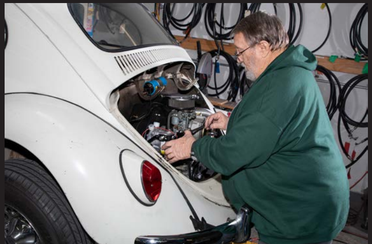
This system uses a single belt, adjusting tension is done by adding or removing alternator/generator shims.
