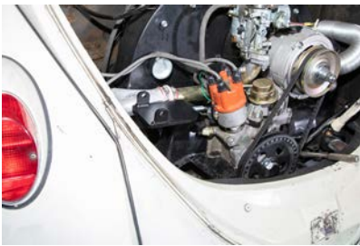
Frank drills a 1 ¼ inch hole in the front engine cover plate tin for the rear compressor brace; a special nut is provided.
