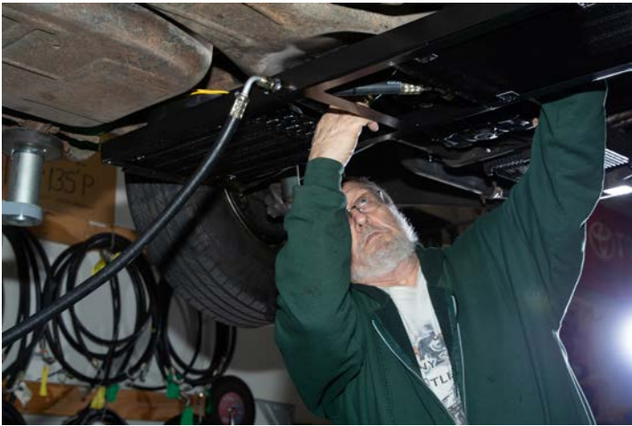
Hoses are attached to the condenser under the car.
