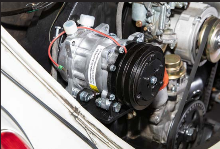
The A/C compressor is mounted to the bracket.
