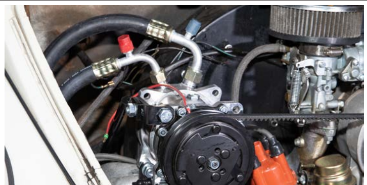
High-pressure hoses are fed from the engine compartment through the tin and attached to the compressor.
