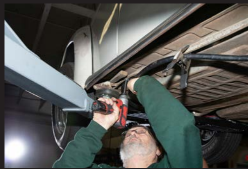
Before affixing the pressure hoses to the body, the original body seal nails must be removed one-by-one using a grinder. The hoses can then be attached using clamps along the channels.
