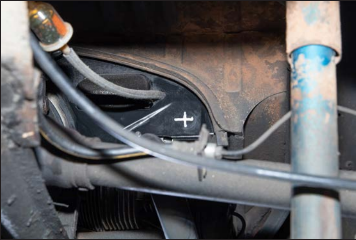
Frank drills a 1 ¼ inch hole in the front engine cover plate tin for the rear compressor brace; a special nut is provided.
