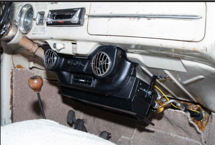
Final wiring for the evaporator is completed, and cork tape is wrapped on the metal fittings of the unit.
