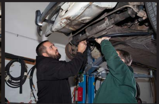
Before affixing the pressure hoses to the body, the original body seal nails must be removed one-by-one using a grinder. The hoses can then be attached using clamps along the channels.
