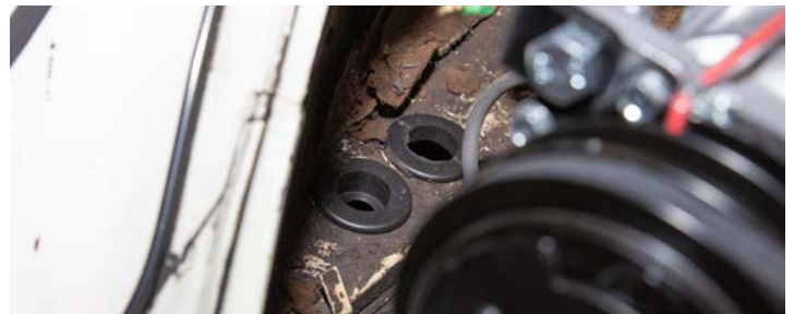
Two 1 ¼ inch holes are needed on the left side of the engine compartment for hose access. These are protected with grommets.
